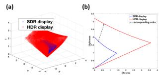
**Figure 3.** (a) the color gamut of both the HDR display and the SDR display and (b) the principle of the HDR gamut mapping approach.
