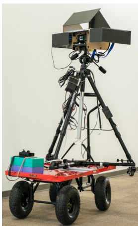
Figure 3. The data acquisition device install on a tripod while the trolley is used for outdoor manoeuvre.
