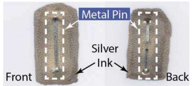
(a) Interconnection made by metal pin from an office stapler
