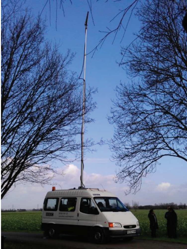
Figure 12: BBC R&D survey vehicle with elevated mast at 10 m Photo: Mark Waddell
