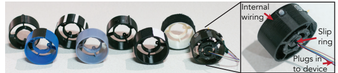
Figure 5. Interchangeable haptic wheels allow applications to customize the haptic experience with various shapes and textures. (right) Wheels with active components use a slip ring in the wheel mount to wire the electronics in the wheel back to the device.
