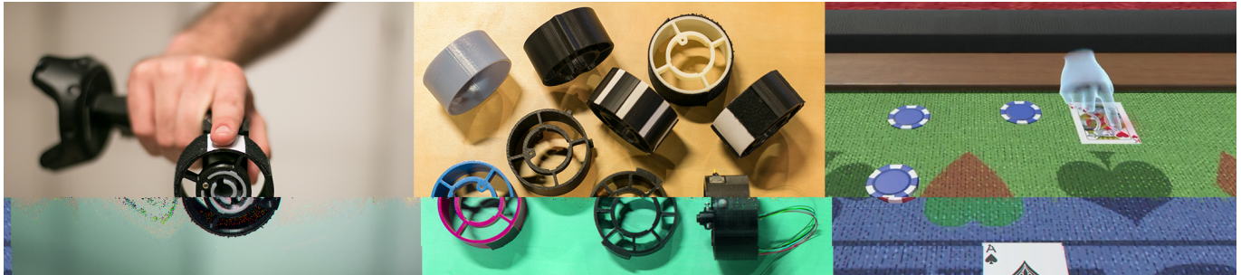
Figure 1. (left) Our Haptic Revolver device uses a wheel that raises and lowers and spins underneath the fingertip to render various haptic sensations. (center) The haptic wheels are interchangeable and can be customized to render arbitrary textures, shapes, or interactive elements. (right) Wheel features are spatially registered with the virtual environment, so the user can reach out and feel virtual surfaces.
