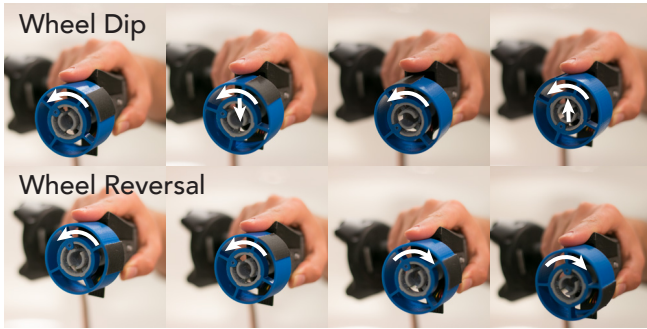
Figure 8. (top) As the finger approaches an obstacle (indicated here by the black region on the wheel), the dip strategy causes the wheel to lose contact with the finger while an undesired feature remains under the finger. (bottom) In the reversal strategy, the wheel begins to rotate in the opposite direction when an undesired feature is encountered.
