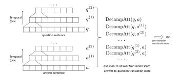
Figure 7: Architecture of the proposed model. DecompAtt stands for a decomposable attention model that is applied to a pair of representations.
