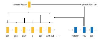
Figure 8: Illustration of the attention-based sequence-to-sequence model.
