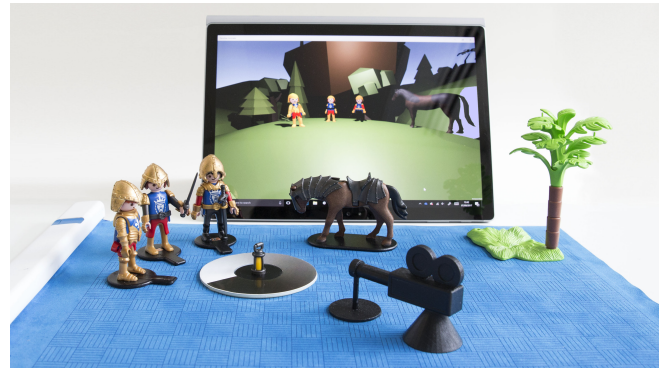
Figure 6. Movie Maker can be used to create video stories by manipulating physical toys. Camera and light props are used to frame and light the scene, which is displayed on a connected device.
