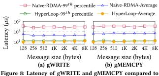
Figure 8: Latency of gWRITE and gMEMCPY compared to Naïve-RDMA.
