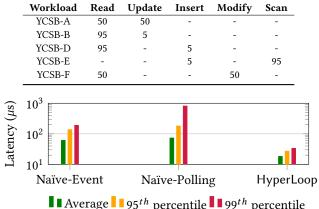
Figure 11: Latency distribution of replicated RocksDB using Naïve-RDMA (event-based and polling) and HyperLoop.
