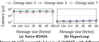
Figure 10: 99<sup>th</sup> percentile latency of gWRITE with different group sizes compared to Naïve-RDMA.
