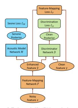
Figure 2: The framework of SA-AFM for speech enhancement. where S is a sequence of senone labels  $S = \{s_1, \ldots, s_T\}$ aligned with the noisy data X and enhanced data  $\hat{Y}$ .
