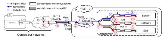
Figure 1: The example scenario. We collect per-hop traces in our network (Y and ISP-Y-switch) and do not have the traces outside our network except the ingress and egress of ISP-Y-switch. The packet format of each numbered network segment is listed in Table 1.
