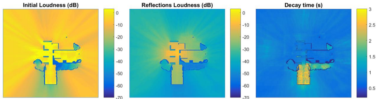
Figure 2. Perceptual parameter fields on the “Cliff House” scene (horizontal 2D slice of 3D field).
