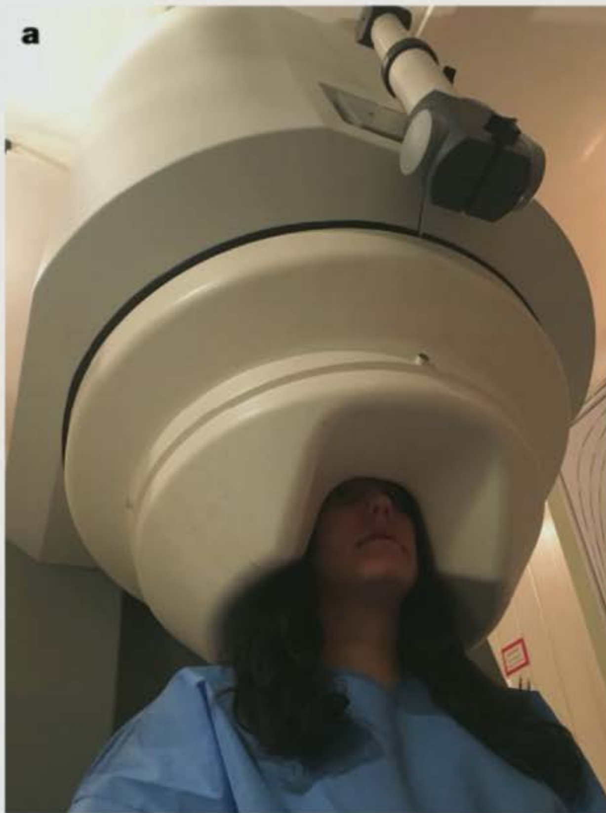
Current MEG scanner based on SQUID sensors
