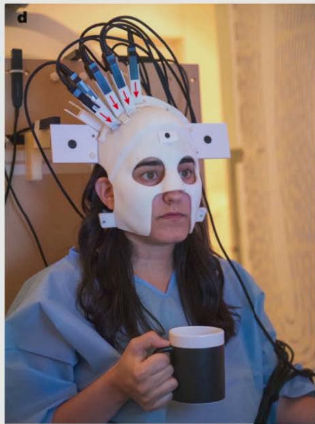
New MEG scanner with OPM sensors
