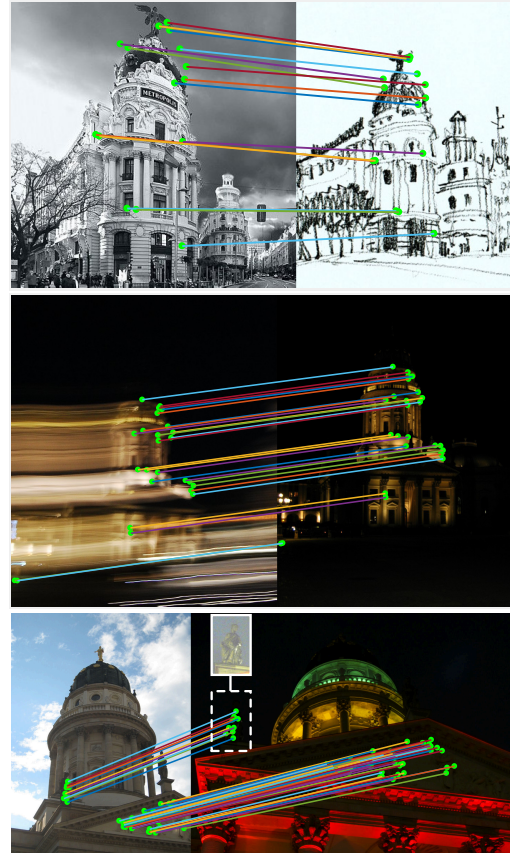
Figure 1: Examples of matches obtained by the D2-Net method. The proposed method can find image correspondences even under significant appearance differences caused by strong changes in illumination such as day-to-night, changes in depiction style or under image degradation caused by motion blur.
