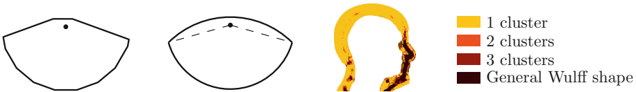
Fig. 3. (Left) 2D illustration of a discretized Wulff shape, where all the training data lies close to a single direction. (Middle) our approximation of the general shape with a surrogate parametric Wulff shape composed out of a spherical sector with an attached spherical cap. (Right) Slice through the volumetric shape prior that indicates the type of Wulff shape used at each place.
