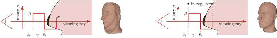
Fig. 2. Unary term for a ray going through the eyebrow next to the skin layer of an example reconstruction (Left) data term of [15]. (Right) our proposed data term. Both sides illustrate the weight added to the voxels along the ray for the class eyebrow by the unary term. (Left) The per-pixel semantic cost \sigma , is entered into the last voxel of the uncertainty region. In this case eyebrow is visible in the image but the weight ends up inside the skin layer due to the very little thickness of the semantic class eyebrow, which leads to artifacts in the reconstruction. (Right) in our proposed data term the weight \sigma is moved to the regularization term. The unary term only captures the geometric information about free and occupied space. This resolves the artifacts in the reconstruction.
