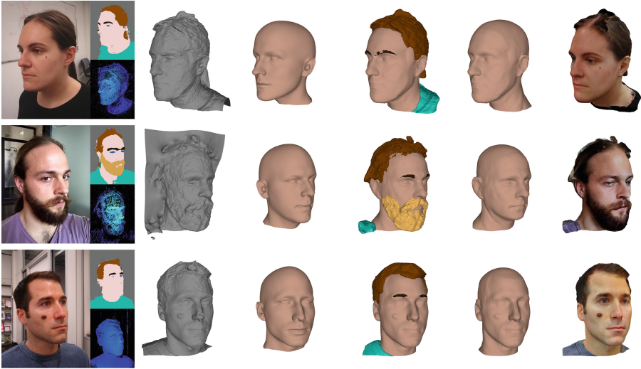
Fig. 5. From left to right: Input image; Input labels and depth; Depth map fusion (TV-Flux fusion from [36]); Statistical model of [23] fitted into our raw input data; Our semantic reconstruction; Our result skin class; Our model textured.
