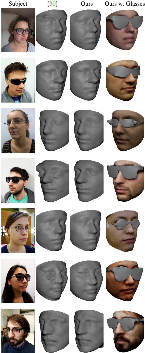
Figure 7: Results for different subjects wearing glasses of various shapes. From left to right: sample input image, result obtained using the method presented in [30], result obtained using the proposed approach, reconstruction of glasses obtained using our approach.
