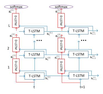
**Fig. 1.** Diagram of layer trajectory LSTM (ltLSTM). Depth-LSTM (D-LSTM) is used to scan the outputs of time-LSTM (T-LSTM) across all layers at the current time step to get summarized layer trajectory information for senone classification. Note that There is no time recurrence in D-LSTM, which only occurs in T-LSTMs.
