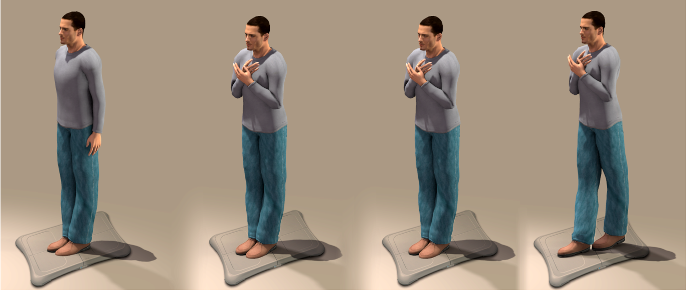
Figure 4. Experiment 2 postures: each subject was recorded in 4 different postures (from left to right): (1) Feet parallel, arms to the side, (2) Feet parallel, arms crossed, (3) Feet parallel, arms crossed, eyes closed (4) Feet in tandem, arms crossed,
