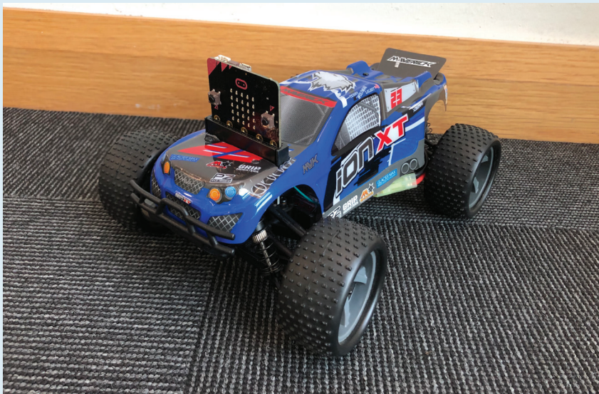
Figure 5. A micro:bit-based vehicle controlled wirelessly by a second micro:bit.
