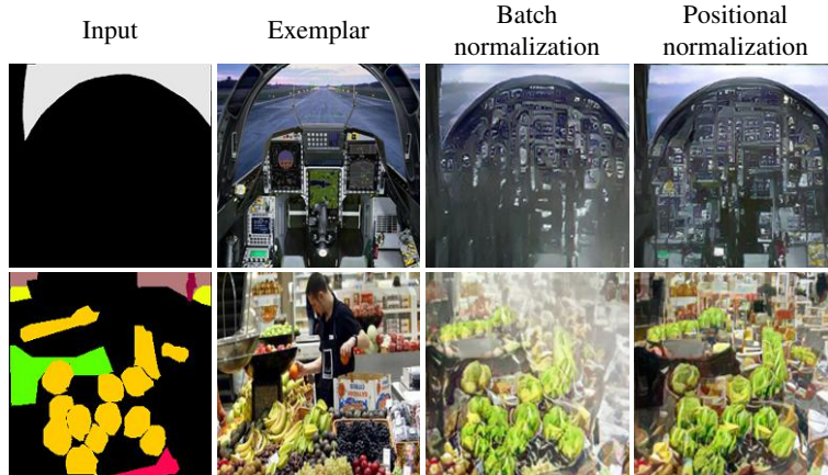
Figure 18: Positional Normalization vs. Batch Normalization. The positional normalization significantly improves the lower bound of the translation image quality.
