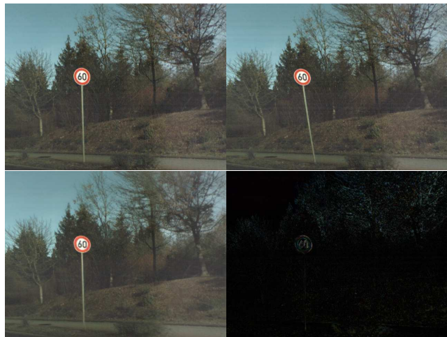
Figure 1: Deep shutter unrolling network. Top left: Ground truth global shutter image. Top right: Input rolling shutter image. Bottom left: Predicted global shutter image by our network. Bottom right: Absolute difference between our predicted image and the ground truth global shutter image.
