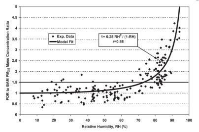
**Environmental Interferences** Non-linear response of particle light-scattering measurements compared to FEM particle matter mass measurements at high levels of relative humidity.
