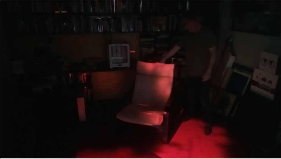
Fig. 4. Projection mapping illustrates areas of the physical environment that have been touched in situ . This includes parts of the chair which have been touched by the person’s hands, as well as areas of the floor touched by the person’s feet.
