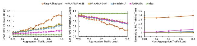
(a) 99%-tile FCT for non-aggregation short (b) Average throughput for non-aggregation (c) Average training time for ML jobs for flows (<40 MB) long flows increasing network load
