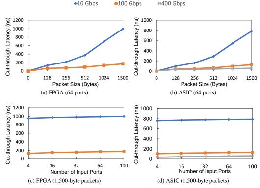
Figure 14: Cut-through latency for different packet sizes assuming 64 ports (a and b) and for increasing number of ports with 1,500-byte packets (c and d).
