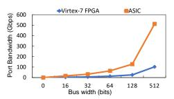
Figure 11: Port bandwidth scaling. Increasing the bus width allows supporting higher port bandwidth.
