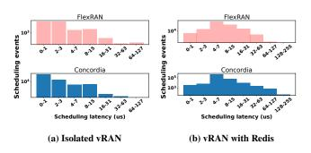
Figure 10: Scheduling latency of vRAN pool worker threads (8 CPU cores) for 2 100MHz cells with and without workload interference (Redis). Y-axis in log scale.
