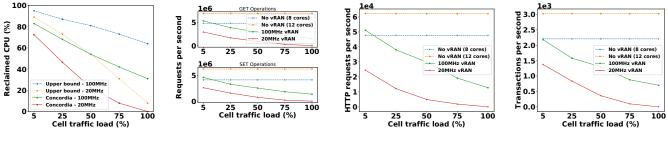
(a) CPU cores reclaimed by Concordia vs ideal case
