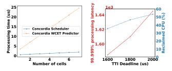
(a) Processing overhead of Concor- (b) Effect of TTI deadline paramdia WCET predictor and scheduler eter on tail latency and reclaimed for a varying number of cells cores (20MHz cell configuration)
