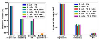
(a) Percentage of slots where the (b) Average WCET prediction erprocessing deadline was violated. ror for successfully met deadline. Y-Y-axis in log scale.
