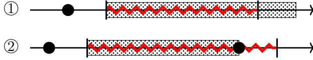
Figure 4: Two typical scenarios supported by mFIT for synchronization between the workload and REF suppression. ● is when the trigger event fires. \color{red}\sim is the time interval when mFIT suppresses REFs, and \text{▨} is the time interval when the workload runs.
