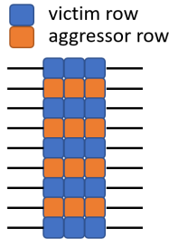
Figure 6: An example of a many-sided attack pattern with 4 aggressor rows and 5 victim rows.
