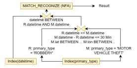
Figure 3: A plan for the query in Figure 1 showing the logical steps to find matches for the pattern (R Z\* B Z\* M).
