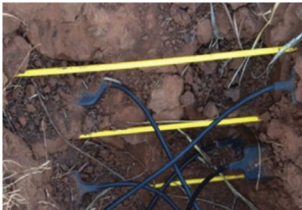
Soil moisture sensors installed next to FO-DTS cables for calibration purposes.
