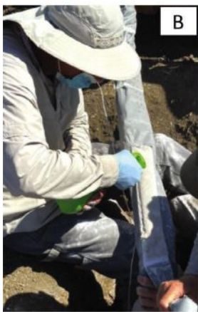
Installation of a deep vadose zone monitoring system (VMS) for continuous monitoring of nitrate leaching to groundwater in a processing tomato field near Esparto, California: (A) insertion of the VMS into the soil, (B) wetting the sampling port prior to insertion into the soil, and (C) the control panel for collecting soil pore water samples.
