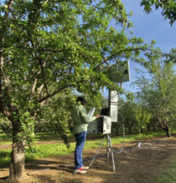
Proximal sensing of orchard-scale soil moisture using a cosmic ray neutron probe in an almond orchard near Corning, California.
