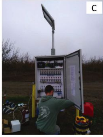
Installation of a deep vadose zone monitoring system (VMS) for continuous monitoring of nitrate leaching to groundwater in a processing tomato field near Esparto, California: (A) insertion of the VMS into the soil, (B) wetting the sampling port prior to insertion into the soil, and (C) the control panel for collecting soil pore water samples.
