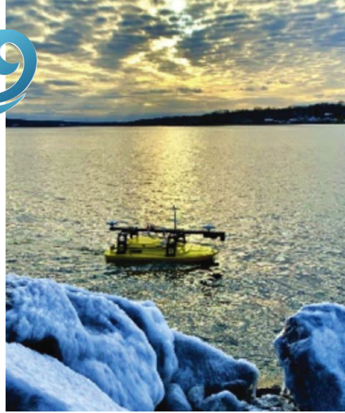
An Echoboat 160 (Seafloor Systems, Inc., Shingle Springs, Calif.) deployed for hydrographic surveying and water quality measurement.
