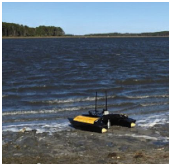
A Heron USV (Clearpath Robotics, Inc., Kitchener, Ontario, Canada) awaiting deployment in an inter-coastal shellfish growing area that is being monitored for potentially harmful concentrations of bacteria.
