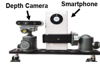
Figure 14: The hardware platform used to evaluate MobiDepth. It aligns the lenses horizontally to guarantee the accuracy of the evaluation.
