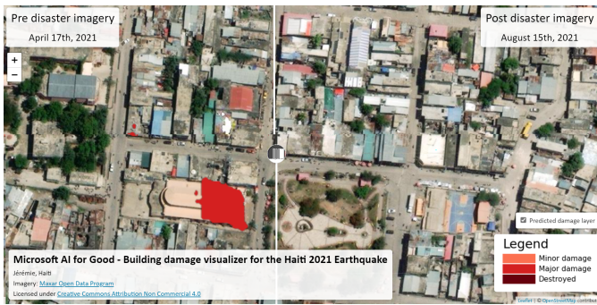
Fig. 6. Screenshot of the building damage visualizer instance for the August, 2021 Haiti Earthquakes. The left side of the map interface shows the pre-disaster imagery while the right side shows the post-disaster imagery. The slider in the middle of the interface allows a user to switch between the pre- and post-disaster layers to quickly see the difference in the imagery. Finally, the building damage predictions are shown as polygons with varying shades of red corresponding to increasing damage. The visibility of these predictions can be toggled in the interface so that a user can see the underlying imagery.
