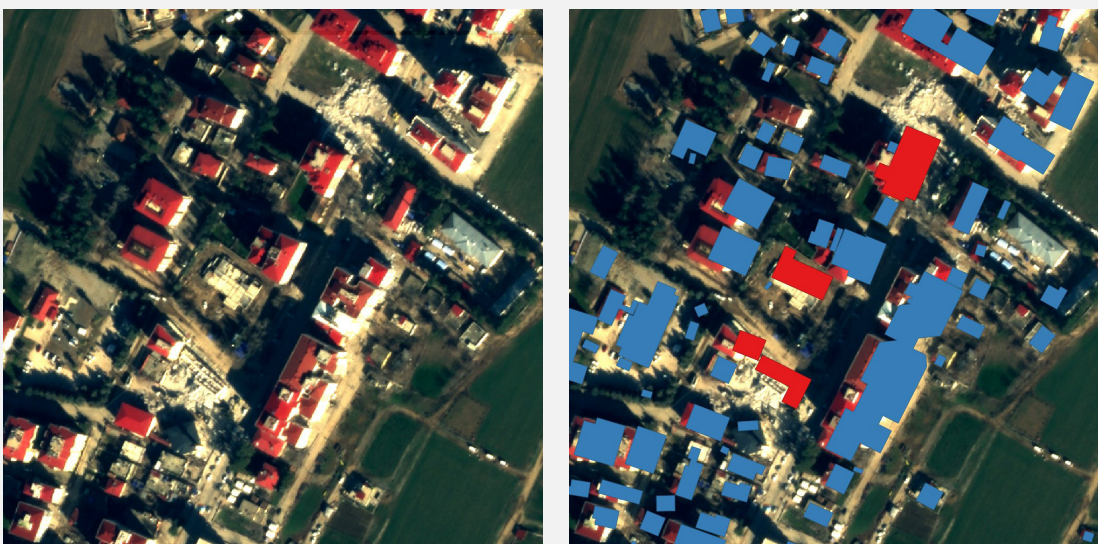
Figure 5: Several destroyed apartment buildings in Turkoglu. Planet Labs PBC, Feb 9th.
