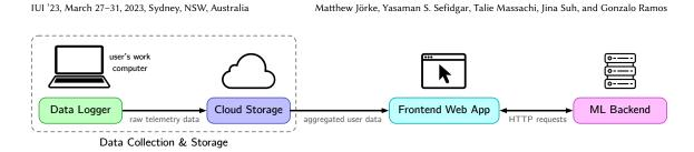
Fig. 2. System Architecture. The data logger runs in the background and records raw telemetry data that is sent to cloud storage. The front-end web application fetches data from cloud storage and sends requests to the ML backend for data featurization and model training.
