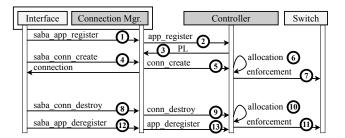
**Figure 7.** High-level overview of interactions between the software interface, the connection manager, the controller, and a network switch.
