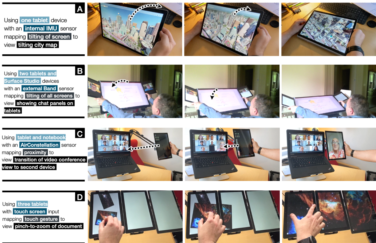
Figure 2: Four examples of designs generated with the Escapement tool. A) A tablet device running both the Sensor Mapper and the Viewer. A tilting motion changes the spatial perspective view of a city. B) A designer attaches an external IMU sensor to a Surface Studio to detect tilt motion. Viewers are open on the Surface Studio, and two additional tablets, which all respond to the tilting motion. The tablets both transition from video content to chat panels as the Surface Studio is tilted down. C) An AirConstellations-enabled tablet [43] allows a designer to use sensed proximity to control the behaviour of a video-conferencing application. D) The Sensor Mapper running on a single tablet (on the left) and an animation split into portions that run on the Viewers on the other two tablets creates the illusion of cross-device zooming via a pinch gesture. Note that all interfaces shown are captured pictures that were ported into the tool - the tool does not interact directly with other applications.
