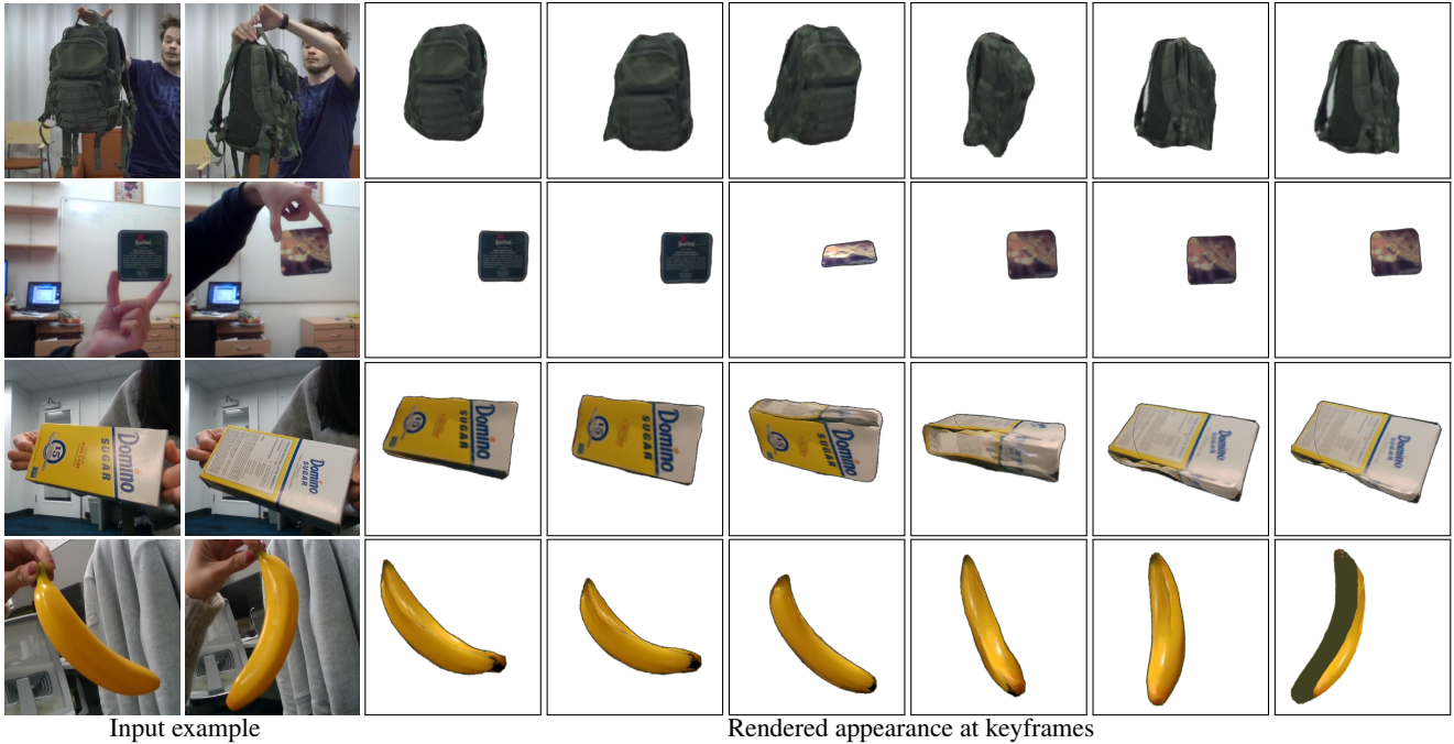
Figure 7. Final 3D textured shape reconstructions. We visualize RGB back-projections (after optimizing with S2DNet [8] features) on a backpack and container sequences from the CDTB dataset [31] (top row), a beermat sequence from the coin tracking dataset [41] (second row), and sugar and banana sequences from [43] (bottom two rows).
