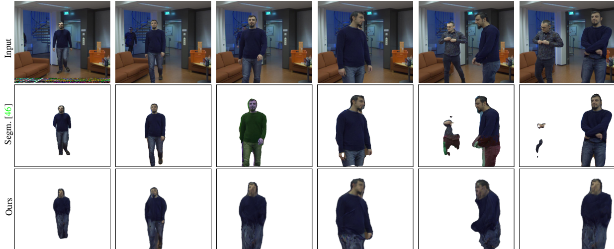
Figure 4. Results with slight non-rigid deformations. Our method successfully reconstructed and improved the segmentation accuracy (by 11.1% IoU on average) on a human body sequence from the CDTB dataset [31].
