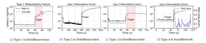
Fig. 6. Four metastability failure types [33] demonstrated in the Blueprint versions of DSB HotelReservation and DSB SocialNetwork.
