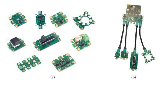
Fig. 1. (a) a variety of Jacdac modules: (first row) light sensor, two different accelerometers, LED ring module; (second row) button, slider, and relay modules ; (third row) passive hub and servo modules; (b) "night light" system—a BBC micro:bit slotted into a Jacdac adaptor, connected to four modules: accelerometer, light sensor, slider, and LED ring.
