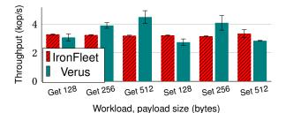
**Figure 10. IronKV Performance.** The Verus version performs comparably to the IronFleet original. Each bar shows the mean of 100 trials; error bars show 95% confidence intervals.
