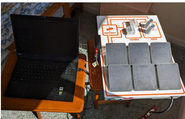
Figure 3: Tabletop Simulator Prototype for a Microgrid
