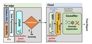
Figure 3: Schematic of SPOTLIGHT system architecture. OOD: Out of Distribution.
