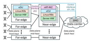
Figure 1: Open RAN defines various open interfaces and consists of hardware and software components provided by diverse vendors (marked in different colors). nRT-RIC: near realtime RIC.
