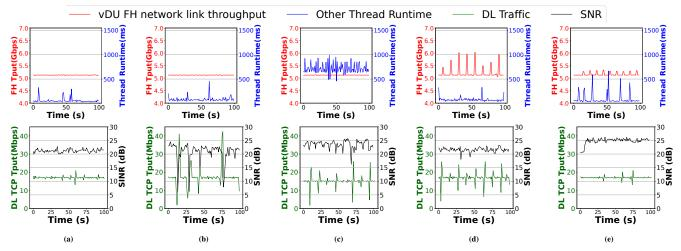
Figure 2: FH link throughput and aggregate runtime of FH related collocated threads (top); DL TCP throughput and SINR at the UE (bottom) for different cases. KPIs for downlink (DL) TCP traffic in (a) normal operation; (b) with external radio interference; (c) with CPU contention on FH thread; (d) with FH network contention; (e) with benign FH network contention.
