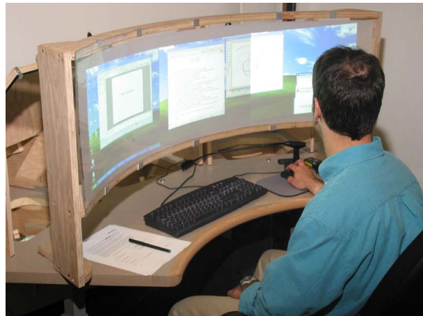
Figure 1. “DSharp” - A Wide Screen Multi-Projector Display
