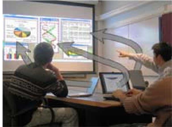
Figure 7. WinCuts used to send portions of two personal laptops to a shared large display.
