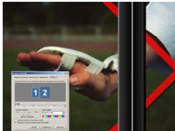
Figure 6. OneSpace used to eliminate distortion in image across a bezel.
