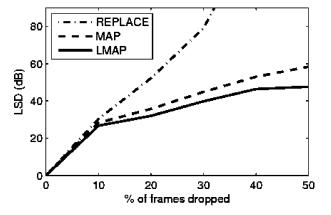
Fig. 2. LSD between original and reconstructed frames for REPLACE, MAP, and LMAP techniques.
