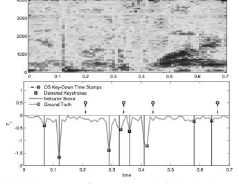
Fig. 1. Top: spectrogram of an utterance corrupted with keystrokes. Bottom: value of  $F_t$  for this utterance. The ground-truth locations of the keystrokes are shown by black solid vertical lines.
