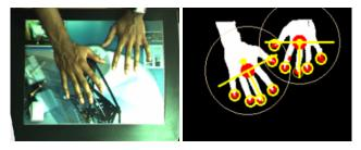
Figure 2. Fingertip detection and multi-touch sensing using stereo vision. (*left*) Input image from one camera after homography transformation; (*right*) Segmentation mask showing orientations of each hand and detected finger tips (bold circles indicate touch).
