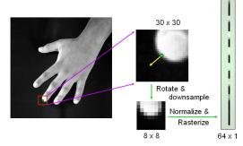
Figure 3. Encoding process that converts each point on the boundary of a hand into a signature vector. These are used to classify each edge-point as a *tip* or *non-tip* point, which are then spatially clustered to locate individual finger tips.
