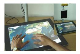
Figure 1. Our multi-touch sensing mechanism allows for enhanced gesture based interactions with an ordinary tablet display, simply by using an overhead stereo camera. The high precision is critical to giving the feel of a real touch-screen.
