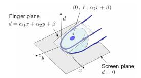
Figure 4. Geometric model of a finger on the screen-plane. The orientation and height of a finger is summarized by a plane computed from the detected tip points; and the surface of the finger tip is well-approximated as an ellipsoid to detect instances of touch.
