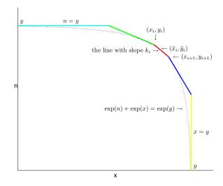
**Fig. 2.** Illustration of the piecewise linear approximation (PLA) of the explicit distortion model.
