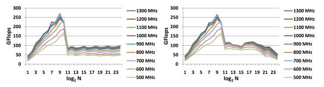
Fig. 10. Varying memory clock rate on the GTX280. The FFTs are performed in shared memory for  $N \in [2, 2^{10}]$ . For  $N > 2^{10}$  we show the performance of the global memory algorithm (left) and the hierarchical algorithm (right). The FFT becomes compute bound for higher memory clock rates, especially for larger sizes in the shared memory kernel.
