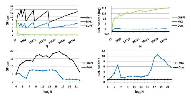
Fig. 16. 1D Prime FFTs. (Top) Performance for batched 1D FFTs, where  $N \in [2^5, 2^{16}]$  is prime. The saw tooth shape of the plot for our FFTs and MKL's is characteristic of the Bluestein algorithm. CUFFT uses an  $O(N^2)$  algorithm which is very slow for large N. (Bottom) Batched 1D FFTs where N is the largest prime not greater than  $2^i$  for  $i \in [1, 24]$  and M = E/N, where  $E \approx 2^{24}$ . For large prime N, our FFTs are up to 10 times faster than MKL.
