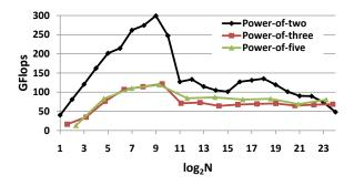
Fig. 18. **Comparison of batched 1D FFT with varying radix**-*R*. Power of two sizes use combinations of radix-2, radix-4, and radix-8. We use only radix-3 and radix-5 for the other cases. Performance could be improved by radices larger powers of 3 and 5. These performance numbers were obtained using a GTX280 with driver version 177.11.
