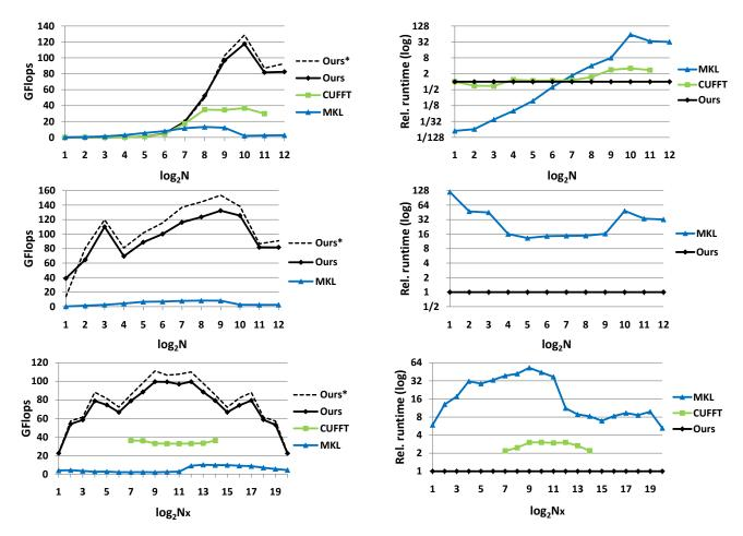
Fig. 14. **2D power-of-two FFTs.** (Top) Performance for single 2D FFTs of size  $N \times N$ . (Middle) Performance for M 2D FFTs of size  $N \times N$ , where  $M = E/N^2$  and  $E = 2^{24}$ . CUFFT not shown because it does not support batched 2D FFTs. (Bottom) Performance of a single 2D FFT of size  $N_x \times N_y$  where  $N_x N_y = 2^{24}$ . CUFFT currently only supports 2D FFTs with  $N_x, N_y \in [2, 2^{14}]$ . The dashed line is for performance on an older driver.
