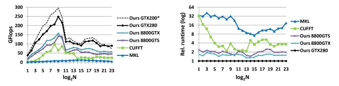
Fig. 12. Batched 1D power-of-two FFTs. (Left) Performance of our algorithms on multiple GPUs, CUFFT on the GTX280, and MKL. The dashed line is for performance on an older driver. (Right) Run time relative to our algorithms on GTX280 (zoomed on large values of N). The number of FFTs M is chosen as E/N, where  $E = 2^{23}$ , the largest value supported by CUFFT. For large N on the GTX280, our FFTs are up to 4 times faster than CUFFT and 19 times faster than MKL.
