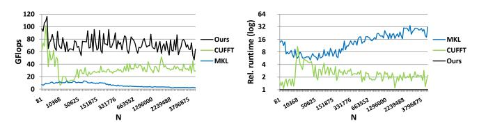
Fig. 15. 1D Mixed-radix FFTs. (Left) Performance for batched 1D FFTs where  $N = 2^i 3^j 5^k$ ,  $i, j, k \neq 0$ , M = E/N, and  $E \approx 2^{24}$ . (Right) Run time relative to our algorithms. For large N, our FFTs are typically 2–8 times faster than CUFFT and 5–32 times faster than MKL.
