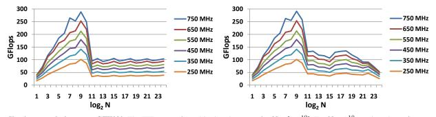
Fig. 9. Varying core clock rate on GTX280. The FFTs are performed in shared memory for  $N \in [2, 2^{10}]$ . For  $N > 2^{10}$  we show the performance of the global memory algorithm (left) and the hierarchical algorithm (right). The global memory algorithm shows small oscillations due to use of radix-2 and radix-4 for the last iteration. The performance of the hierarchical algorithm drops off as N increases. For all but the smallest sizes, performance scales linearly with clock rate.
