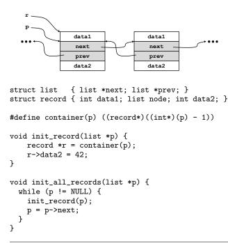
Figure 1. Example C code. The diagram shows two record structures in a linked list, with the embedded list shown in gray.
