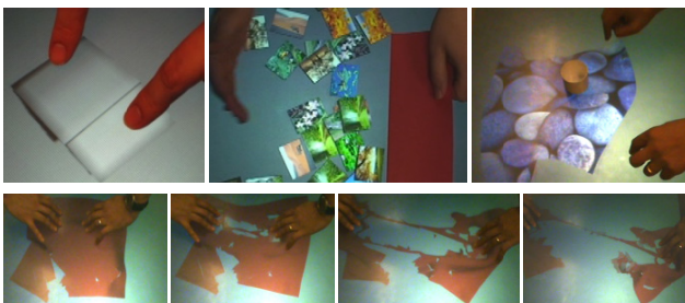
Figure 7. A cambered card is slid on top of another by pushing one side while holding the bottom card in place (top left); tangible objects interact with the digital: e.g., the side of a physical piece of card used to gather up objects (top middle), or a real cup used to pin down a cloth (top right); tearing a mesh in two by applying opposing forces (bottom).
