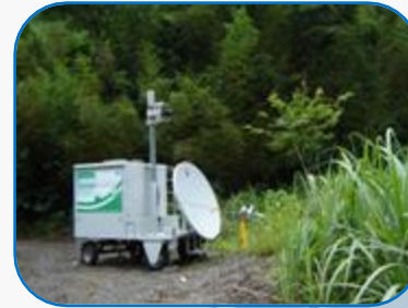
Debris Flow sensor
