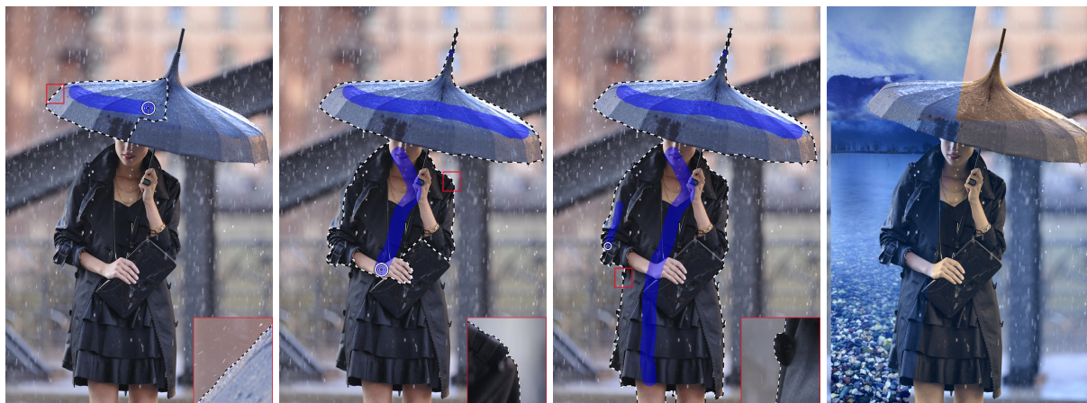
Figure 1: Left three: the user makes a selection by painting the object of interest with a brush (black-white circle) on a 24.5 megapixel image. Instant feedback (selection boundary or image effect) can be provided to the user during mouse dragging. Rightmost: composition and effect (sepia tone). Note that the blue scribbles are invisible to the user. They are drawn in the paper for illustration only.
