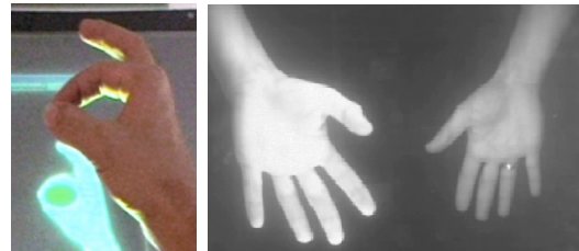
Figure 2 Left: detection of thumb and forefinger pinch gesture. Right: pixel intensity based height estimation.
