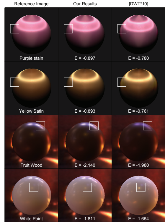
Figure 4: Comparison of the rendering results of reconstructed BRDF with our apparatus and [DWT*10] to the reference rendered with full sampled BRDF. The purple stain and yellow satin are rendered with point light source to show the highly anisotropic appearance. The fruit wood and white paint are rendered with environment map lighting. Note how our method captures the reflectance details on the NDF as well as faithfully reproduces the Fresnel effects near the grazing angle.
